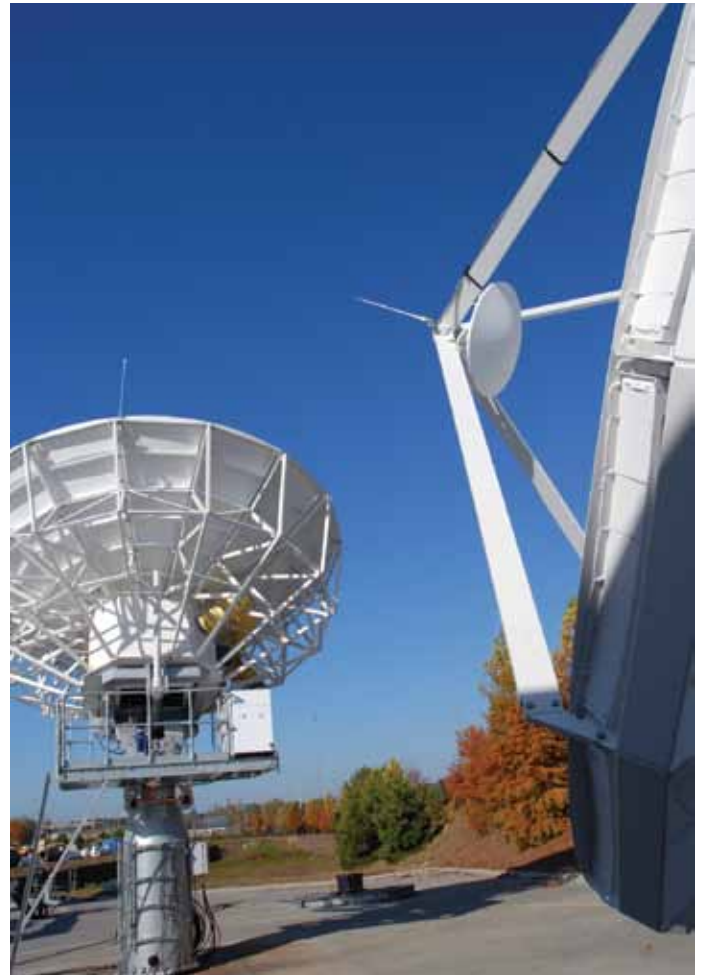
O3b's Tier-1 antenna and gateway terminal in tests at ViaSat in Atlanta
